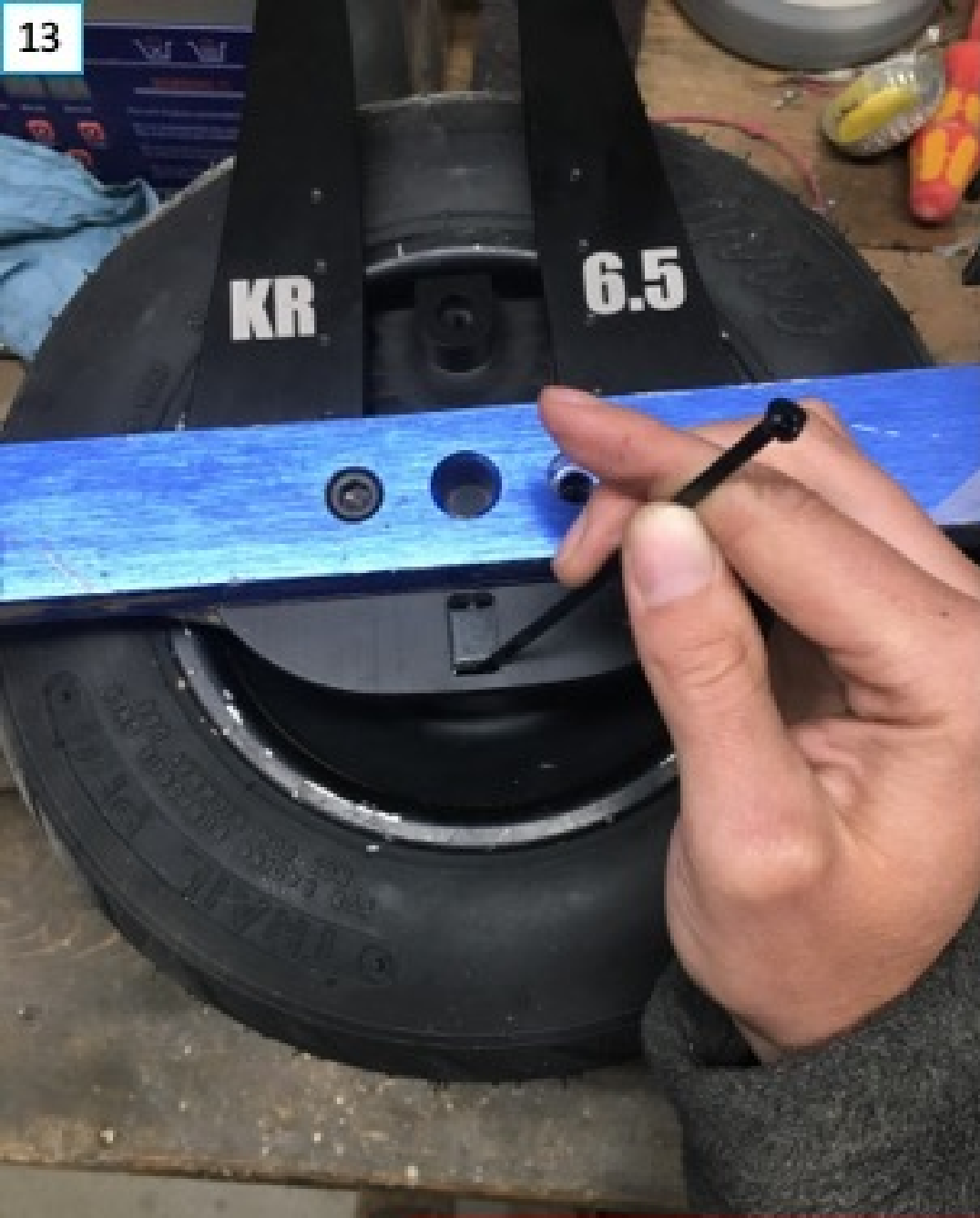
Install the zip tie around your harness to secure it to the tower and trim the excess
